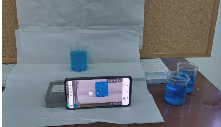
Figure 1. Measuring the parameter H with Color Grab app for android.
