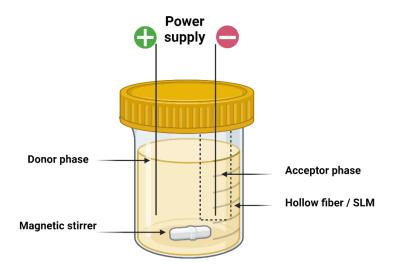
Figure 1 Electromembrane extraction (created with BioRender.com)
