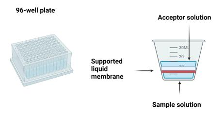
Figure 2 Parallel Artificial Liquid Membrane Extraction (Created with BioRender.com)
