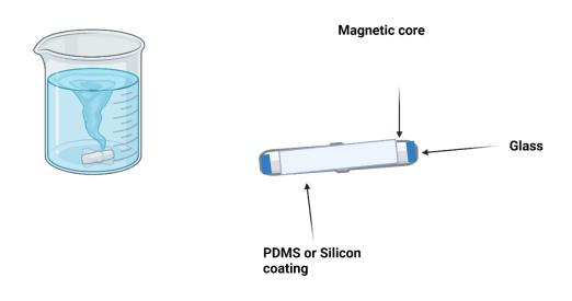
Figure 6 Stir Bar Sorptive Extraction (Created with BioRender.com)
