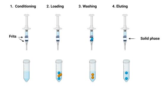
Figure 5 Microextraction by Packed Sorbent (Created with BioRender.com)
