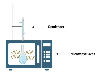
Figure 7 Microwave Assisted Extraction (Created with BioRender.com)
