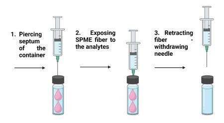
Figure 4 Solid Phase Microextraction (Created with BioRender.com)
